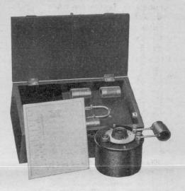
capacitance varies with the setting of the S. L. W. plates, while the circular plates cause no change as they rotate, but act like a fixed condenser. The whole condenser is enclosed in a crackle finished metal can. The spreading of wavelengths by this method is such that one scale division represents about ½ of 1 percent of the wavelength being measured. It is possible to set the scale closer, with care.
